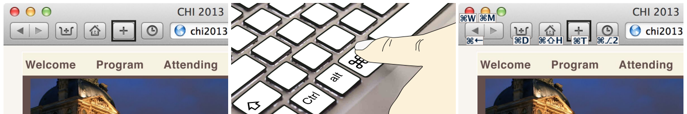
Figure 1. The user wants to open a new tab but is not sure of the hotkey. He visually locates the button in the toolbar (boxed on left), then presses the Command key (⌘) to activate ExposeHK, which overlays toolbar items with available hotkeys (right). He completes the command by pressing ⌘T.
