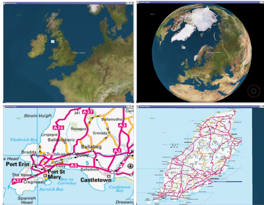
Figure 2. The automatic-zooming globe interface at slow (left) and high (right) speeds in the globe-view (top), and at slow and high speeds in the city view (bottom).
