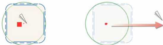
Figure 4: Lens dismissal. A stylus that moves quickly from inside to out "breaks" the lens' boundaries and dismisses it.
