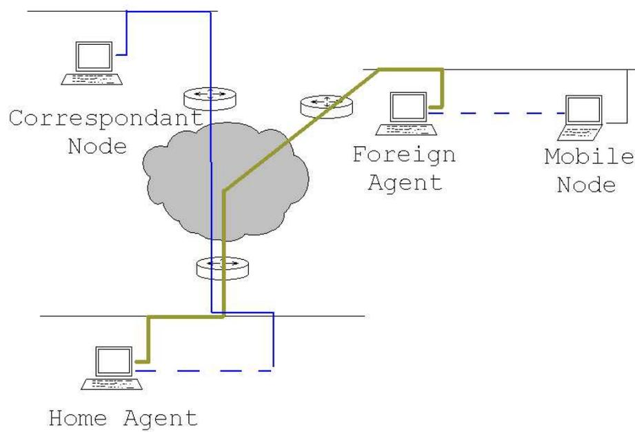
Figure 2: Mobile IP routing using a foreign agent and reverse tunneling
