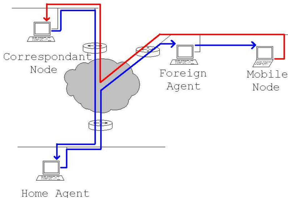
Figure 1: Mobile IP routing using a foreign agent and triangular routing
